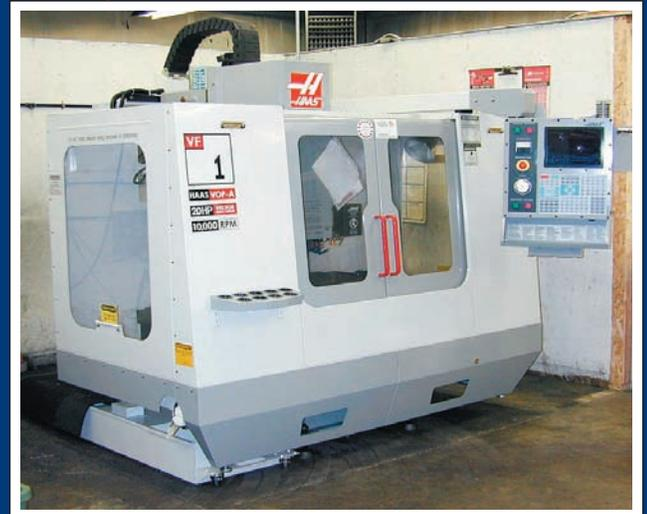
Our CNC machining operations are streamlined using Haas vertical machining centers. The CNC machining capabilities provide a powerful tool to reduce cycle times and improve accuracy. Our machining centers are equipped with 20-station tool changers. One machining center is equipped with a 10,000 RPM spindle. With our CNC machining centers we are capable of quickly and accurately meeting the needs of the tool and die and production machining industry.
