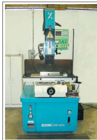
Our small hole EDM can burn holes in carbide and steel ranging from .5mm (.020") to 3mm (.118") diameter in a short amount of time. The Drillmate EDM is tooled with Gaiser, 3R and Hirshman tooling.
